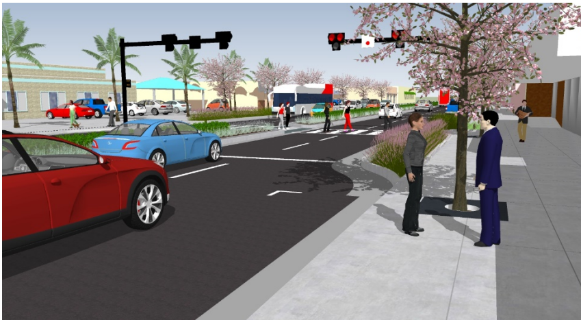
Example of traffic calming utilizing a protected crosswalk, bulbouts and a center median to slow traffic speeds, improve pedestrian visibility and enhance the aesthetic of the area. Photo source: Michael Baker International
