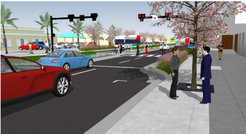
Pedestrian crossing with a Pedestrian-actuated Hybrid Beacon (PHB). This device is extremely effective in stopping vehicles for pedestrian crossings where regular traffic signals are not warranted. Photo source: Michael Baker International
