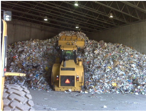
Example of a solid waste transfer station.
